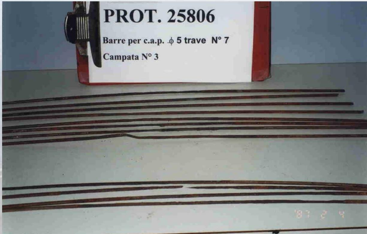
Colajanni, P., Recupero, A., Ricciardi, G., Spinella, N. - Failure by corrosion in PC bridges: A case history of a viaduct in Italy (2016) *International Journal of Structural Integrity*, 7 (2), pp. 181-193
