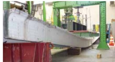
Failure of the control unstrengthened TT beam
