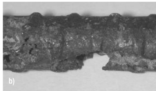
Figure 1. Examples of the effects of corrosion of steel in concrete: (a) spalling of the concrete cover due to carbonation induced corrosion, (b) localised attack on a bar due to pitting corrosion in chloride contaminated concrete.
