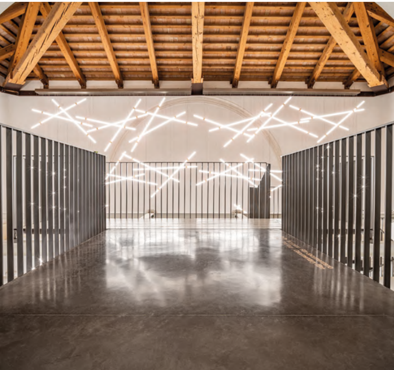
Ca' Scarpa - Treviso (TV) SKYCONCRETE® INDOOR Finitura lucida/ 2 mm. Ca' Scarpa - Treviso (Italy) SKYCONCRETE® INDOOR Glossy finish/ 2 mm.
