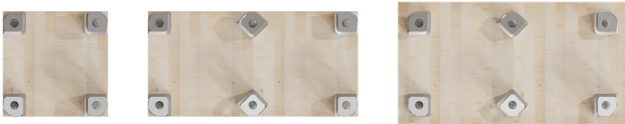
Figure 3. Arrangement of ROOCO® Column Shoes in different column cross-sections.
