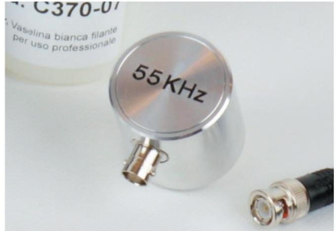
Figure 3 - Dettaglio sonda TX/RX a 55 kHz
